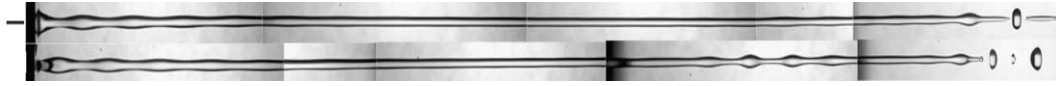
Fig. 7. Image of water-glycerol mixture jet discharging from the elliptical orifice E4 at We = 39.26 . All other details remain same as in the caption of Fig. 4.
